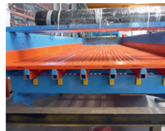
Side protection strips (made of plastic, rubber or highly wear-resistant steel)
