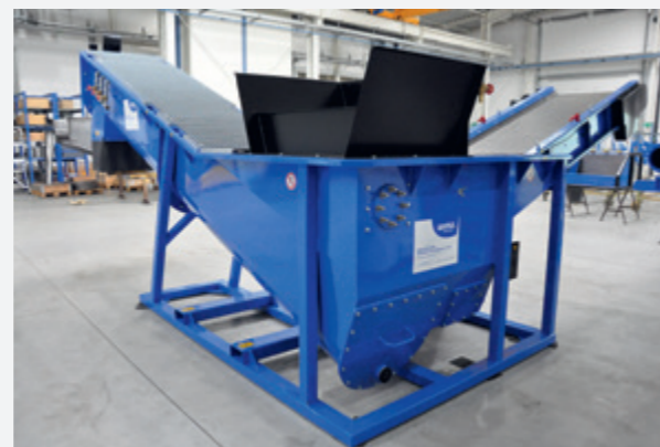
HDS-S view: feed hopper and maintenance door
