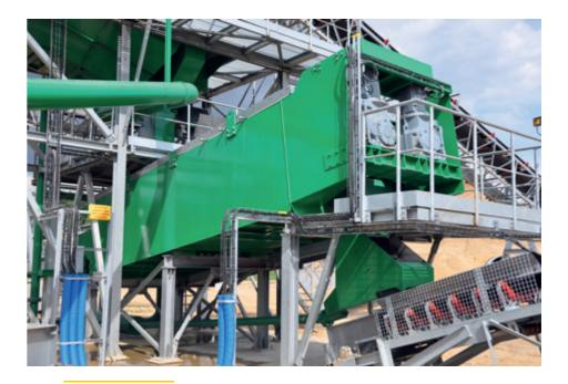
The WIMA Twin Shaft Log Washer discharges the purified material through a Curved Screen below the DWSW onto a conveyor belt for dewatering.
