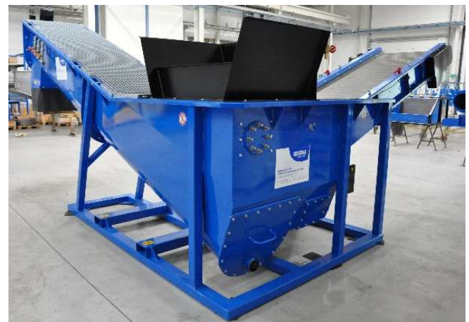
HDS-S view on feed hopper and service openings
