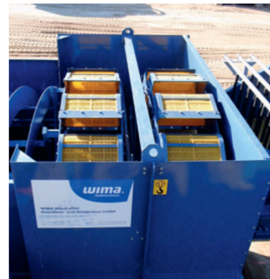
DES model with washing wheel, bucket wheel and Dewatering Screen Machine
